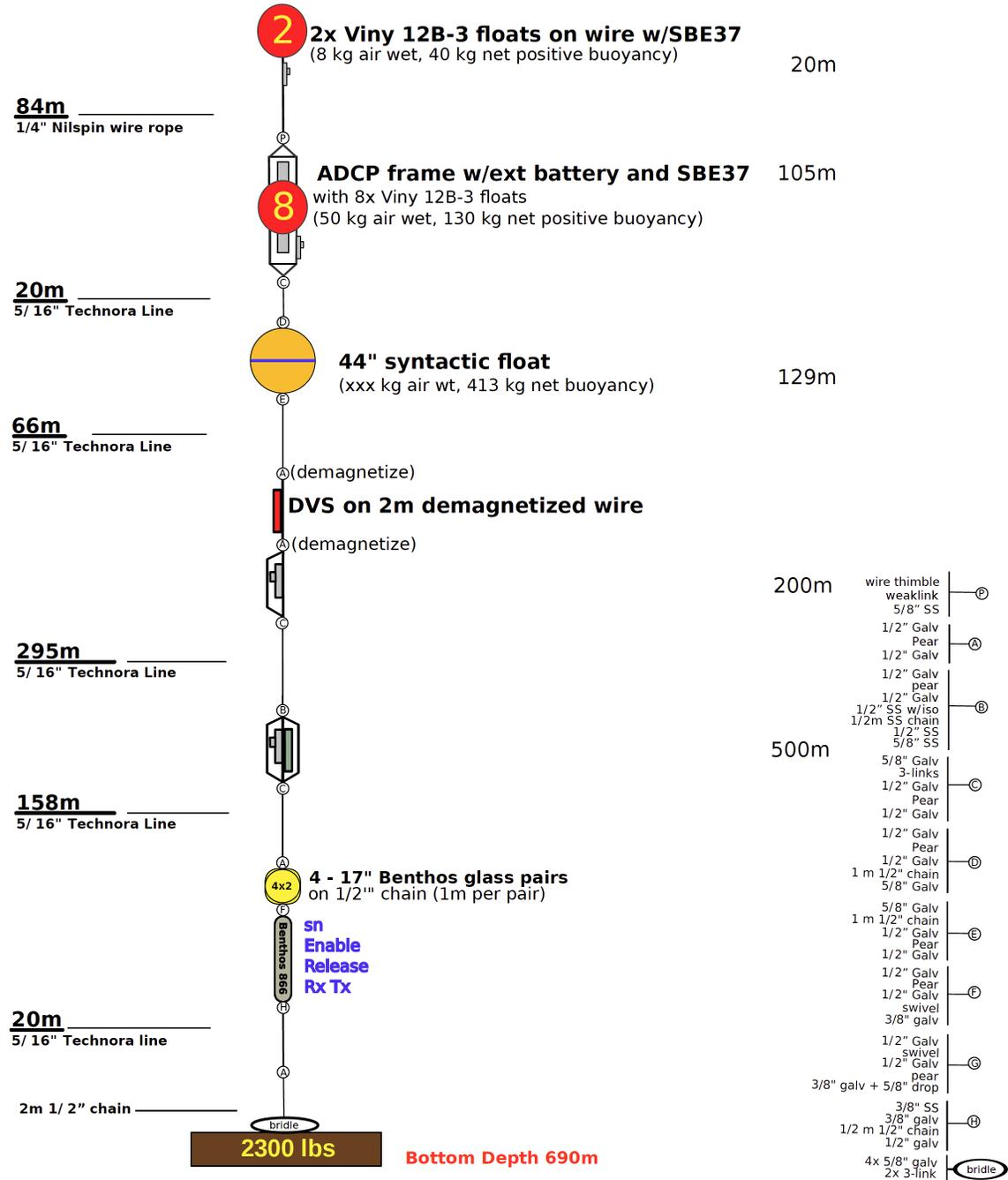
Figure 4k. C5 Mooring diagram (central strait).
