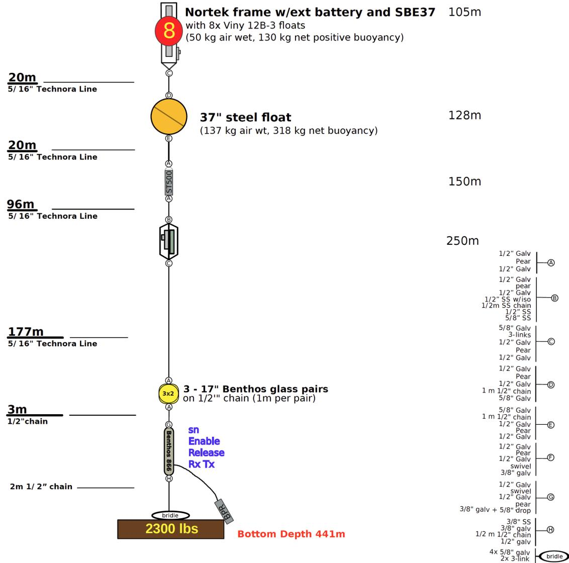
Figure 4g. C1 Mooring diagram (central strait).
