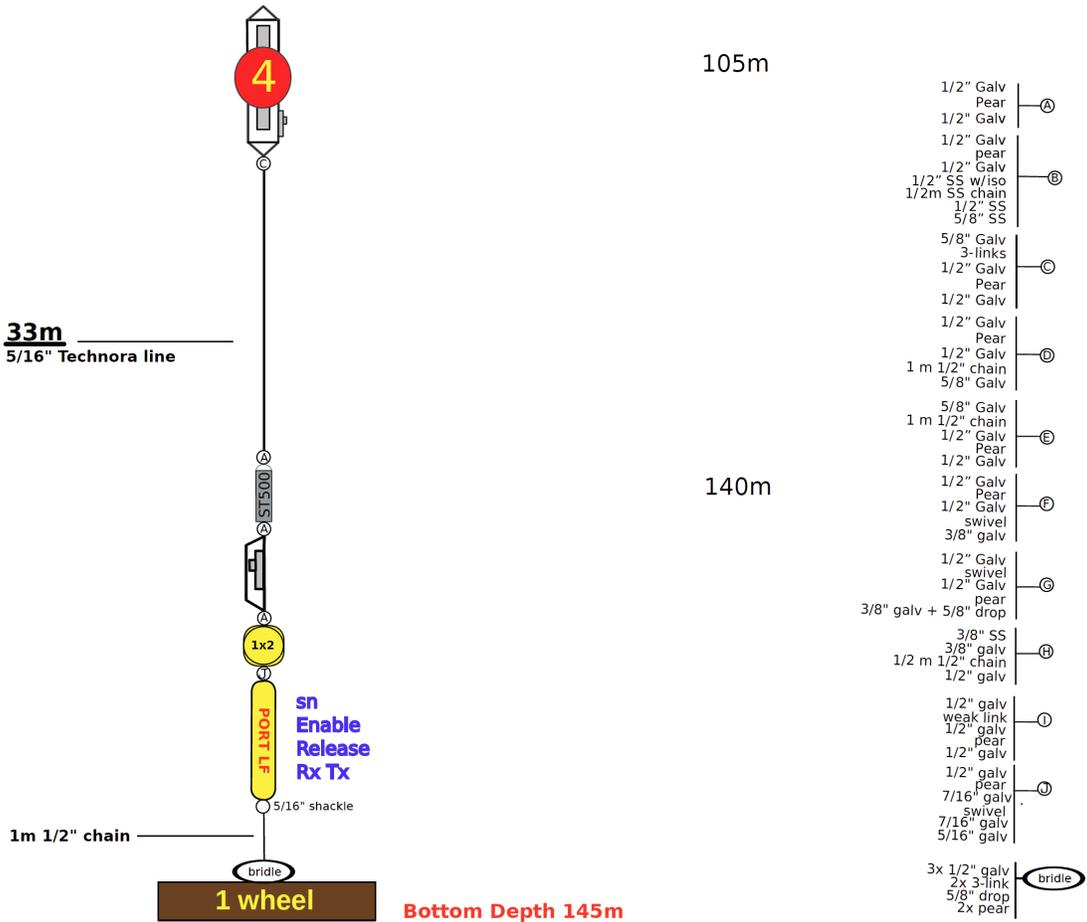
Figure 4c. WG1 Mooring diagram (West Greenland Shelf).
