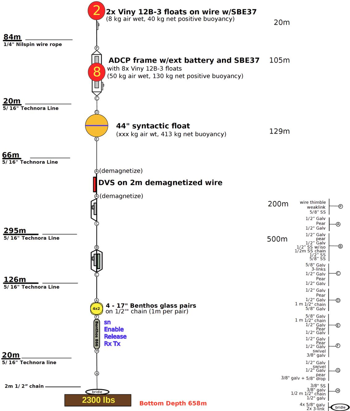
Figure 4h. C2 Mooring diagram (central strait).
