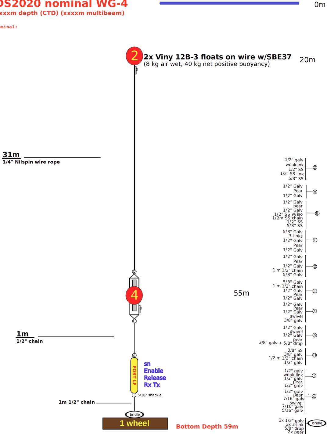
Figure 4f. WG4 Mooring diagram (West Greenland Shelf).
