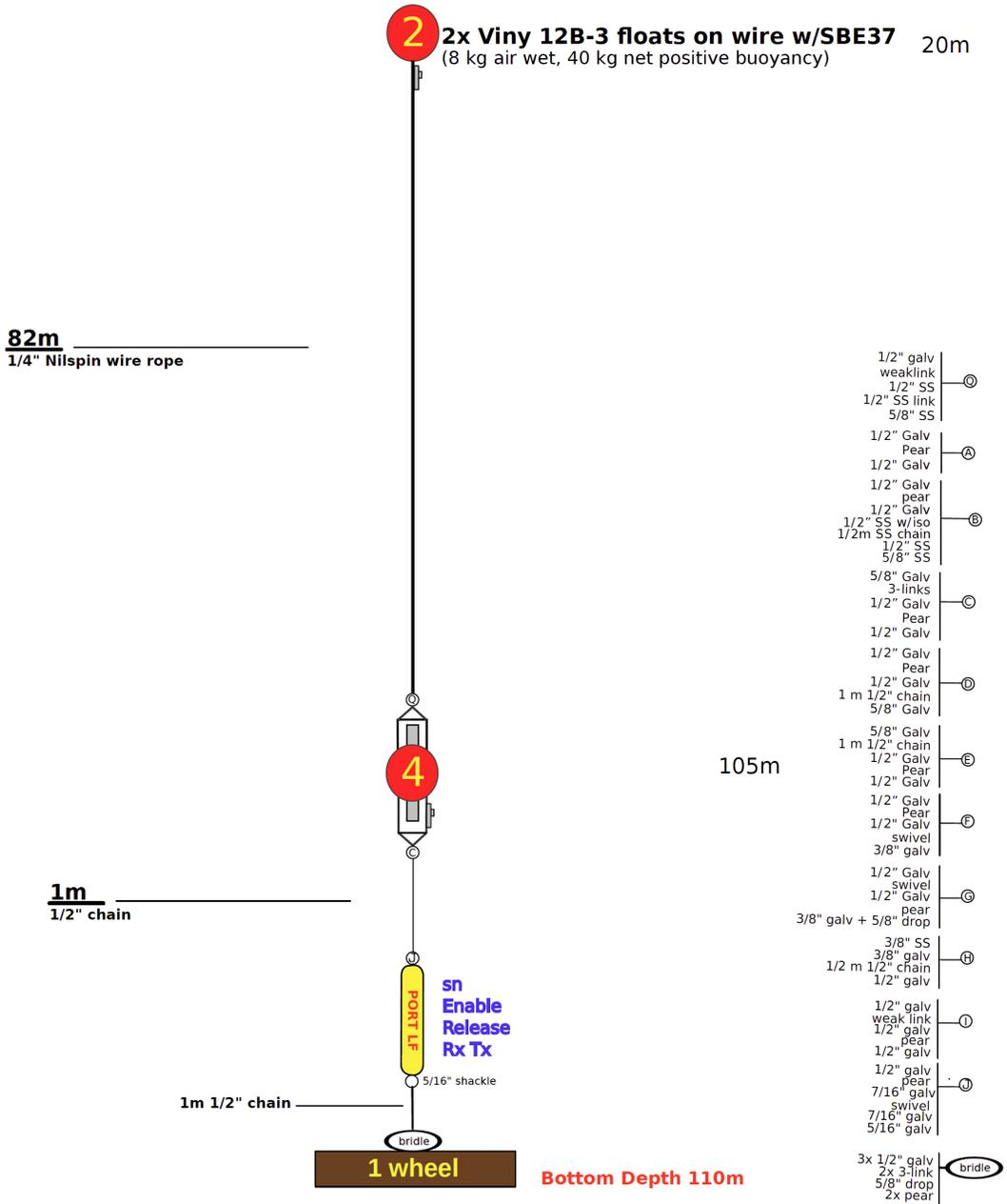
Figure 4d. WG1.5 Mooring diagram (West Greenland Shelf).
