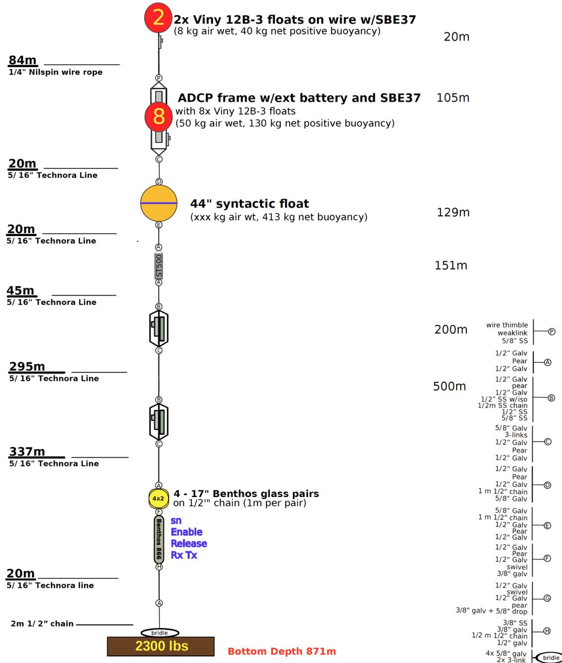
Figure 4j. C4 Mooring diagram (central strait).
