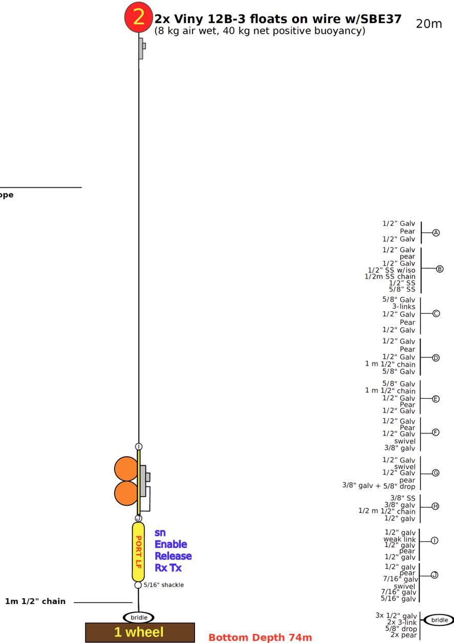
Figure 4e. WG2 Mooring diagram (West Greenland Shelf).
