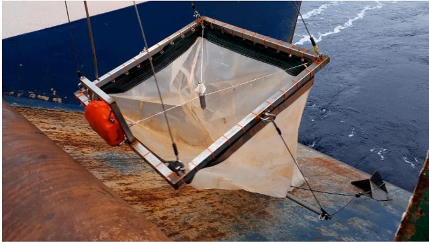
**Figure 6.** Single square net (SSN) used to sample age-0 fish and mesozooplankton during the cruise after the loss of the DSN.
