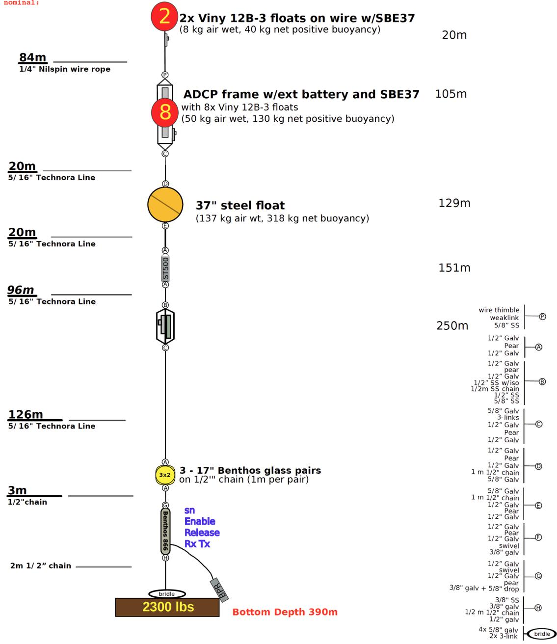
Figure 4l. C6 mooring diagram (central strait).
