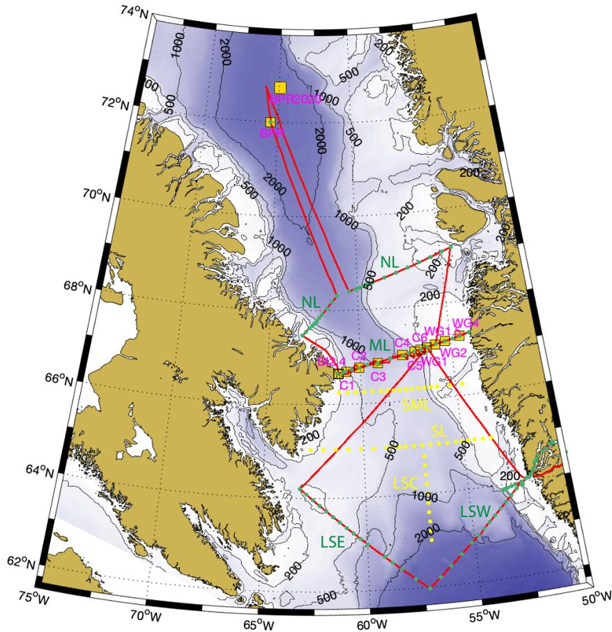
**Figure 2.** Davis Strait mooring sites (orange squares), and standard hydrographic sampling sections: Northern Line (NL), Mooring Line (ML), Labrador Sea West (LSW), Labrador Sea Central (LSC) and Labrador Sea East (LSE). Yellow and green dots mark CTD stations, with green dots indicating those sampled during the 2022 field program. Two previously sampled sections, the South Mooring Line (SML) and Southern Line (SL), are no longer regularly occupied.
