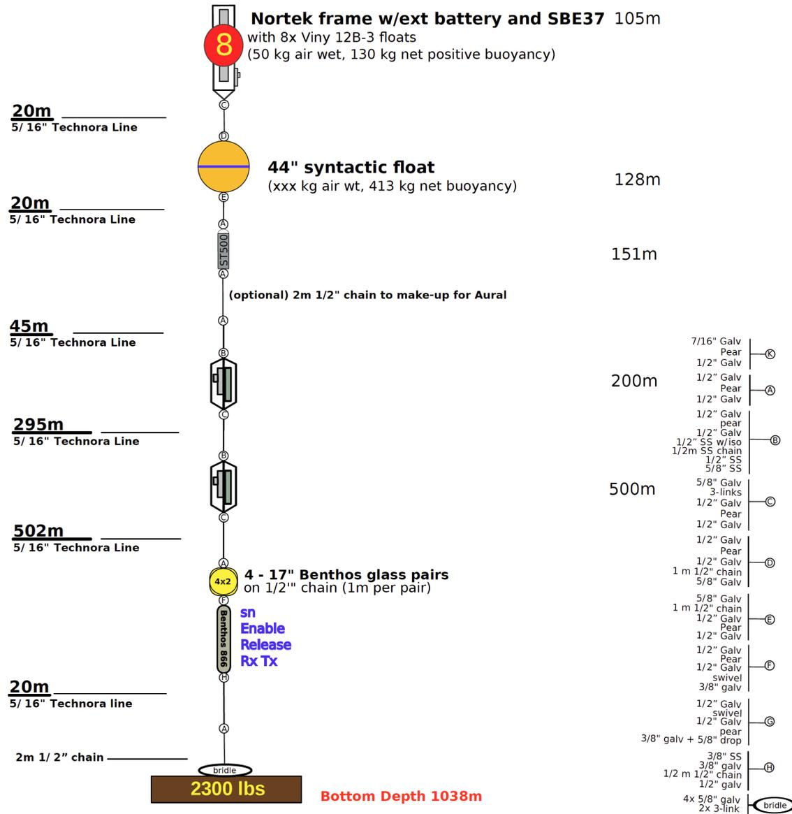
Figure 4i. C3 Mooring diagram (central strait).
