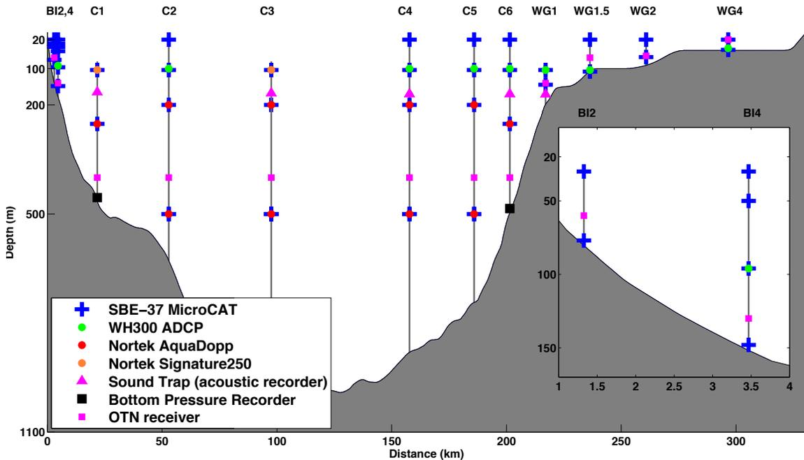
**Figure 3.** The Davis Strait mooring array. Nortek Signature 250-kHz, 5-beam Doppler current profilers (water velocity profile, ice velocity, and ice draft) replace the WH300 ADCPs and IPS ice sonars previously deployed at C2 and C3. NORTEK AquaDopps replace the RCM11 current meters previously used for deeper current measurements.
