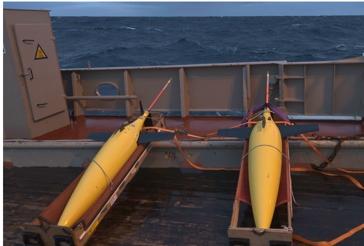
Figure 13. APL-UW ice-capable Seagliders. Gliders are small (50 kg, 1.5 m), long-endurance (multi-month), buoyancy-driven vehicles capable of navigating survey patterns while diving from the surface or ice–ocean interface to depths up to 1000 m. Iridium satellite modems provide two-way communications for command and data upload. Payload includes Seabird T and C, dissolved oxygen, downwelling irradiance, and temperature microstructure.
