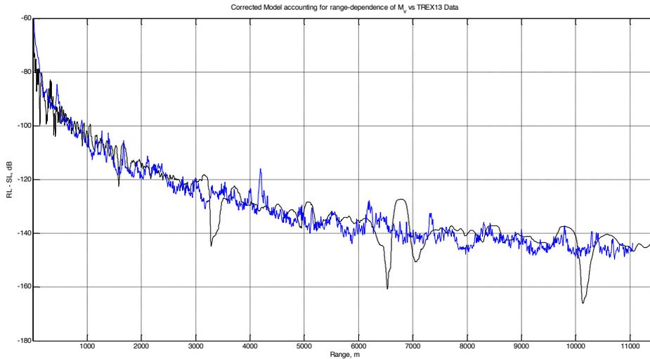
Figure 19: TREX13 normalized reverberation intensity, RL-SL, at 3.4–3.5 kHz, measured after storm (blue), compared to that calculated for volume scattering in sand bottom with corrected range-dependent local volume scattering strength shown in Figure 18.
