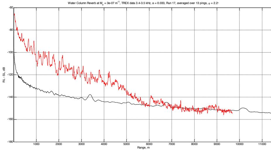
Figure 13: TRES13 normalized reverberation intensity, RL-SL, at 3.4–3.5 kHz, measured before storm (red), compared to model result calculated for scattering in the water column with volume
