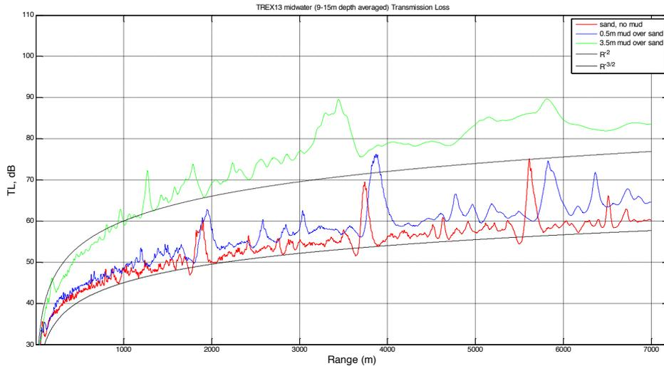
Figure 6: Range-dependence of transmission loss in mid-water, averaged (smoothed) over 100-m span and over 9–15-m depths, 3.5-kHz PE-propagation field in shallow water (20 m depth) for three bottom types: sand half-space (red), 0.5 m of mud over sand (blue), and 3.5 m of mud over sand half-space (green). The source is 1 m above the bottom. Also shown are  $R^{3/2}$  and  $R^2$  range-dependences.
