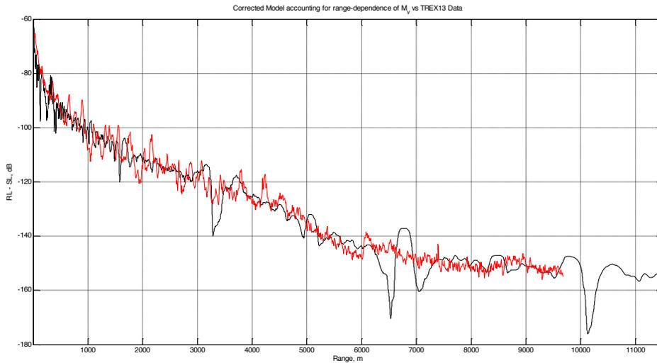
Figure 16: TREX13 normalized reverberation intensity, RL–SL, at 3.4–3.5 kHz, measured before storm, compared to that calculated for volume scattering in a sand bottom with corrected range-dependent volume scattering strength shown in Figure 15.
