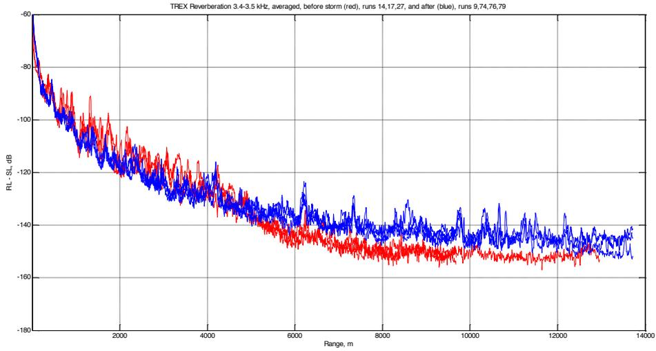
Figure 20: TREX13 normalized reverberation intensity, RL-SL, at 3.4–3.5 kHz, measured before (red) and after (blue) storm. Five more runs added to Figure 12, showing that the previous two runs are typical.
