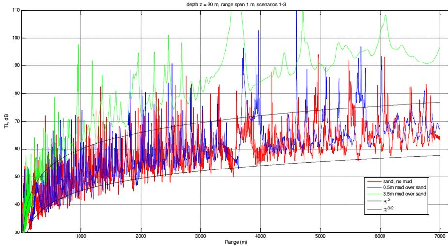
Figure 4: Range dependence of transmission loss at the bottom surface (20 m depth), 3.5-kHz PE-propagation field for three different types of bottom: sand half-space (red), 0.5 m of mud over sand (blue), and 3.5 m of mud over sand half-space (green). The source is 1 m above the bottom.
