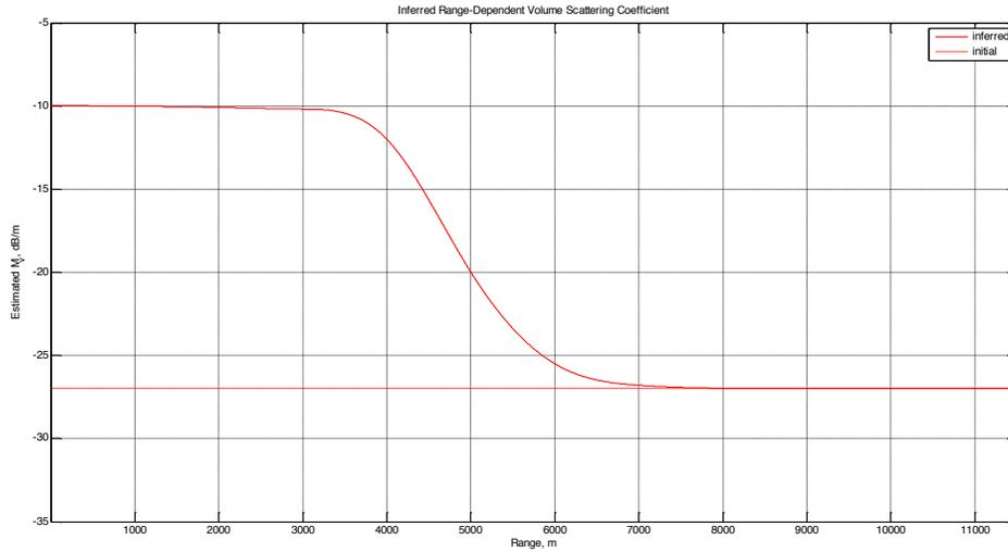
Figure 15: A correction made for range-dependence of local volume scattering strength in the TREX13 sand bottom before a storm.
