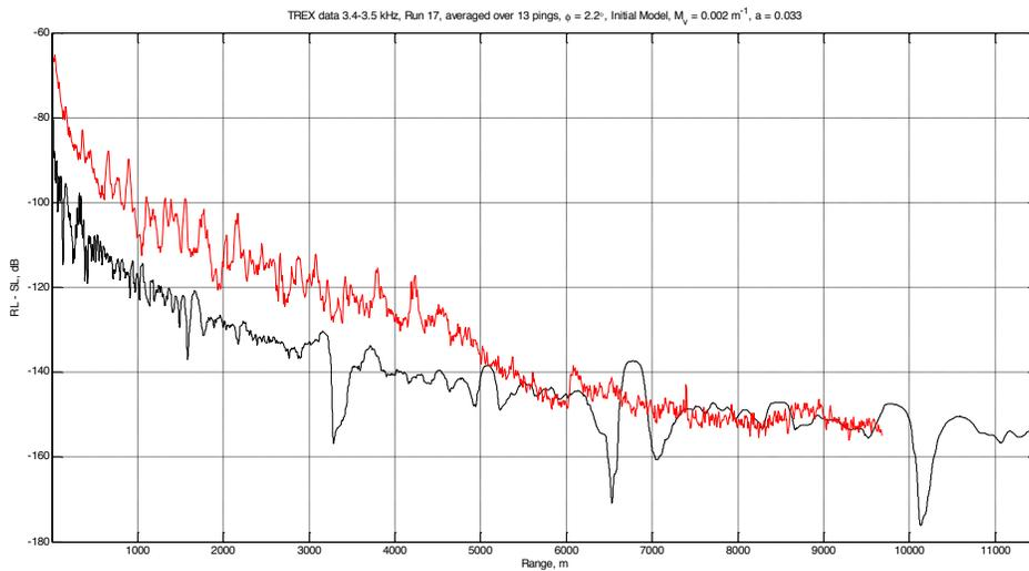
Figure 14: TRES13 normalized reverberation intensity, RL-SL, at 3.4–3.5 kHz, measured before storm (red), compared to that calculated for volume scattering in a sand bottom (range-
