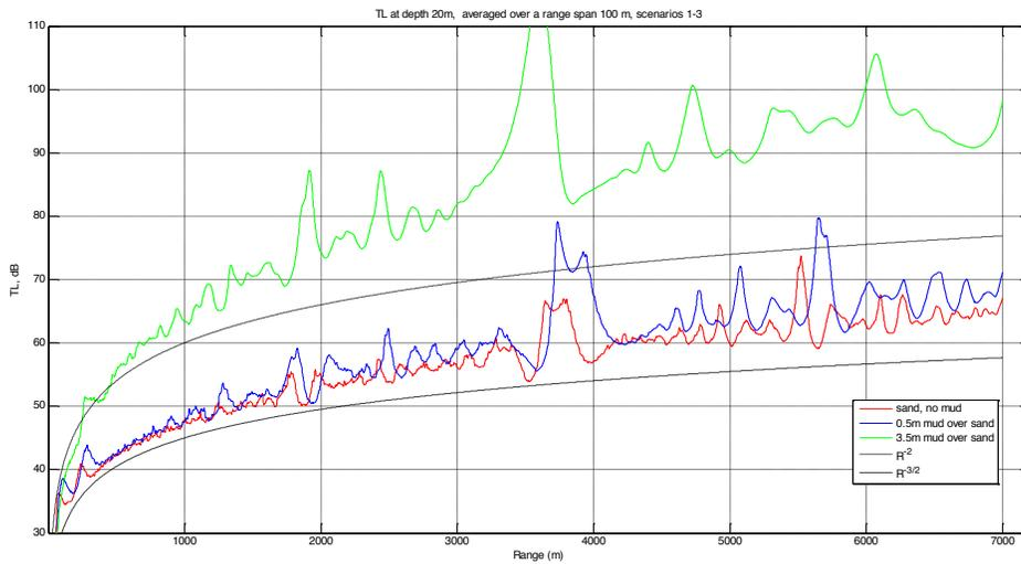
Figure 5: Smoothed 100-m span range-dependence of transmission loss at the bottom surface (20 m depth), 3.5-kHz PE-propagation field for three different types of bottom: sand half-space (red), 0.5 m of mud over sand (blue), and 3.5 m of mud over sand half-space (green). The source is 1 m above the bottom. Also shown are  $R^{3/2}$  and  $R^2$  range-dependences.
