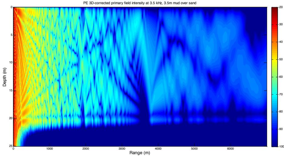
Figure 3: Intensity of 3.5-kHz PE-propagation field in shallow water (20 m depth) with a two-layer, 3.5 m of mud over sand, bottom. The source is 1 m above the bottom.
