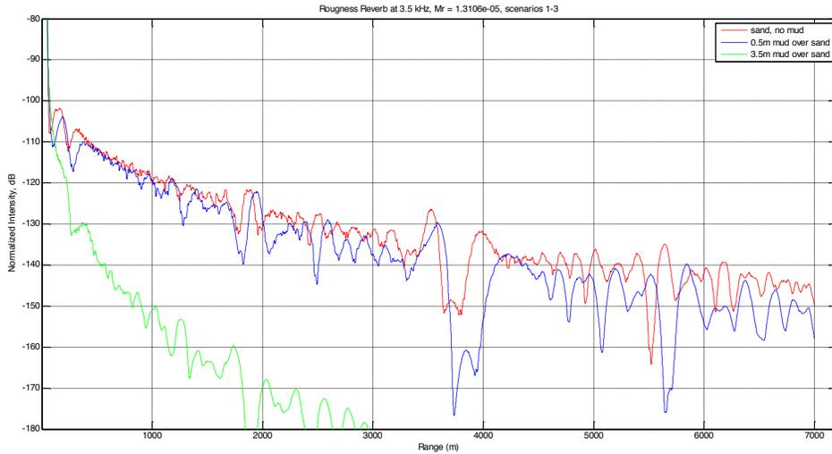
Figure 10: Normalized intensity of reverberation, RL–SL, at 3.5 kHz, caused by bottom interface roughness, with  $M_R = 1.3 \times 10^{-5}$ . Shallow water (20 m depth) with three different types of bottom: sand half-space (red), 0.5 m of mud over sand (blue), and 3.5 m of mud over sand half-space (green). The source is 1 m above the bottom.
