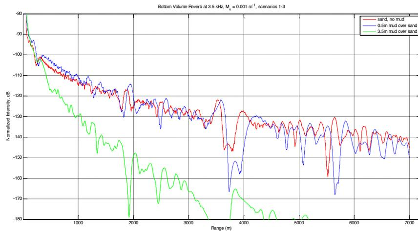
Figure 8: Normalized intensity of reverberation, RL–SL, at 3.5 kHz, caused by sediment volume scattering with  $M_V = 10^{-3} \text{ m}^{-1}$ . Shallow water (20 m) with three different types of bottom: sand (red), 0.5 m of mud over sand (blue), and 3.5 m of mud over sand (green). The source is 1 m above the bottom.
