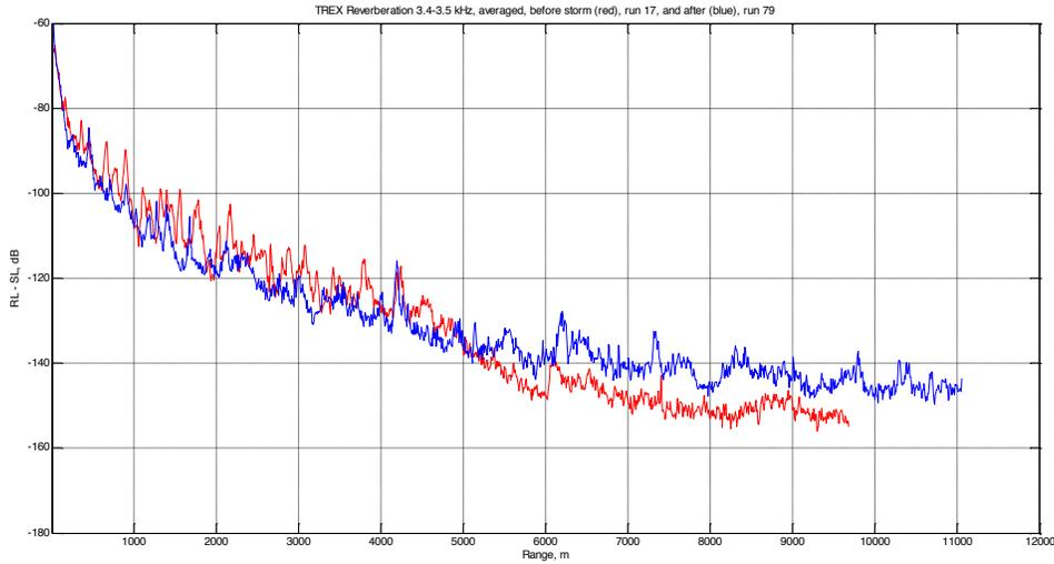
Figure 12: TREX13 normalized reverberation intensity, RL–SL, at 3.4–3.5 kHz, for two runs, before (red) and after (blue) a storm.
