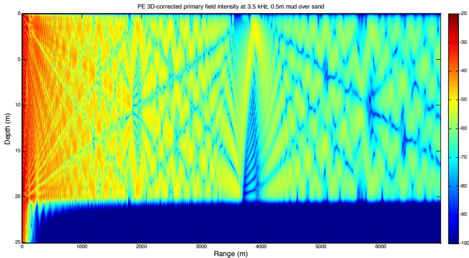
Figure 2: Intensity of 3.5-kHz PE-propagation field in shallow water (20 m depth) with a two-layer, 0.5 m of mud over sand, bottom. The source is 1 m above the bottom.
