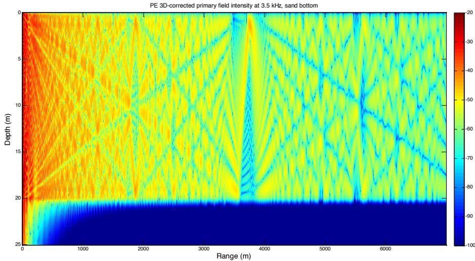
Figure 1: Intensity of 3.5-kHz PE-propagation field in shallow water (20 m depth) with sand bottom. The source is 1 m above the bottom.
