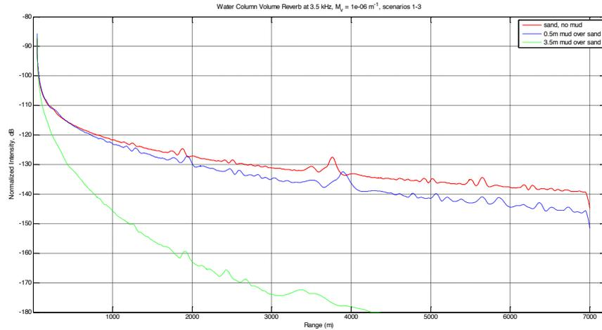
Figure 7: Normalized intensity of reverberation, RL–SL, at 3.5 kHz, caused by volume scattering in the water column with  $M_V = 10^{-6} \text{ m}^{-1}$ . Shallow water (20m) with three different types of bottom: sand half-space (red), 0.5 m of mud over sand (blue), and 3.5 m of mud over sand half-space (green). The source is 1 m above the bottom.
