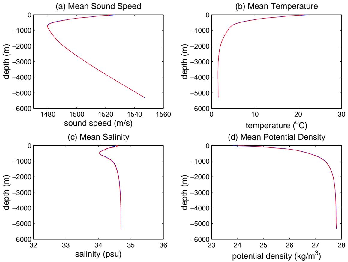
Figure 70. Range-averaged means for IW98 in blue and IW99 in red for (a) sound speed in m/s, (b) primary temperature in °C, (c) primary salinity in psu, and (d) potential density in kg/m<sup>3</sup>.
