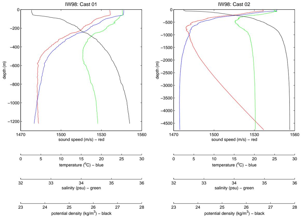
Figure 101. Processed data from Cast no. 1, file name 2280551 (left) and Cast no. 2, file name 2281355 (right) from IW98. Sound speed is in red, temperature is in blue, salinity is in green and density is in black.
