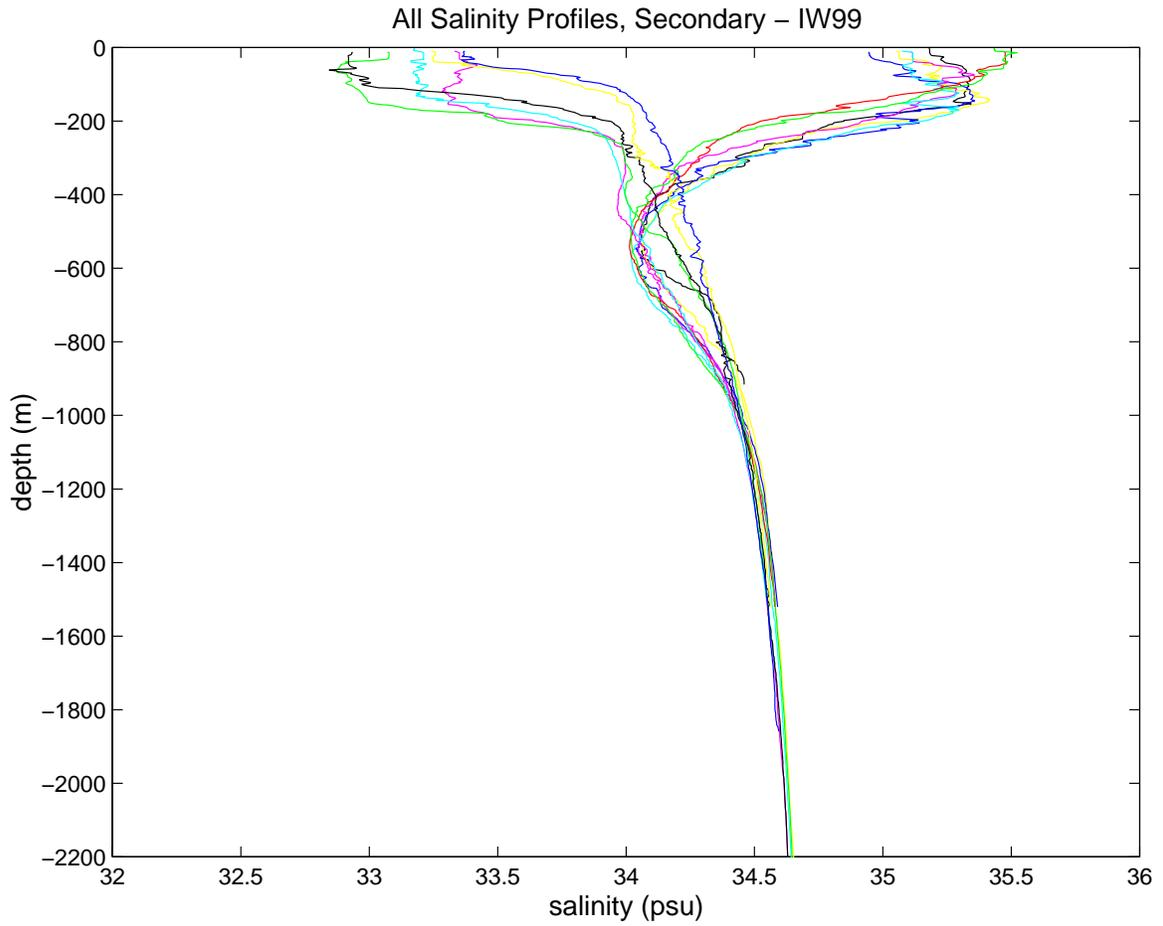
Figure 56. Salinity profiles, in psu, computed from the secondary sensor on IW99 from the surface down to 2200 m.
