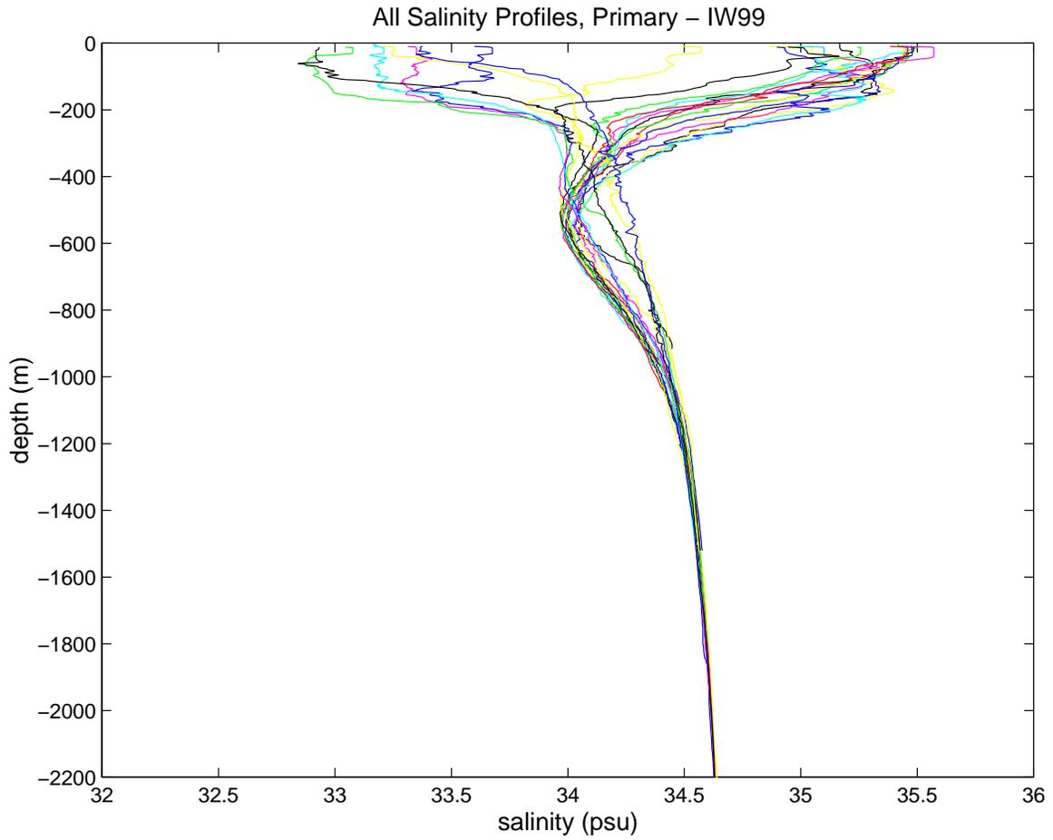
Figure 53. Salinity profiles, in psu, computed from the primary sensor on IW99 from the surface down to 2200 m.
