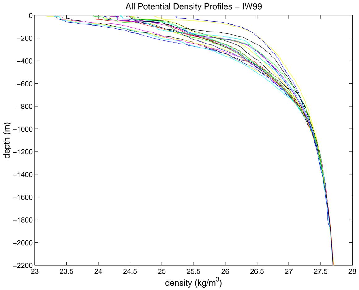
Figure 59. Potential density profiles, in kg/m<sup>3</sup>, from the IW99 cruise from the surface down to 2200 m.
