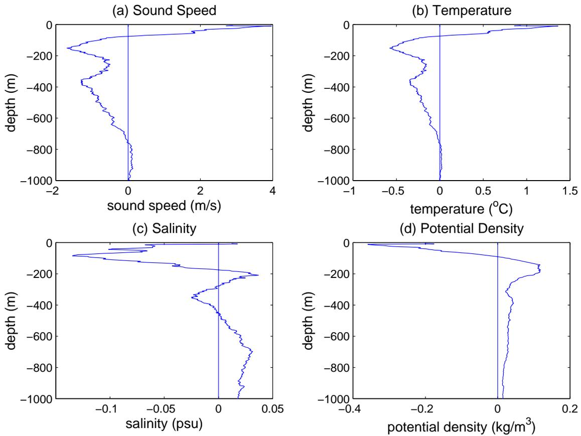
Figure 72. Difference in range-averaged means from IW98 minus IW99 for top 1000 m, for (a) sound speed in m/s, (b) primary temperature in °C, (c) primary salinity in psu, and (d) potential density in kg/m<sup>3</sup>.
