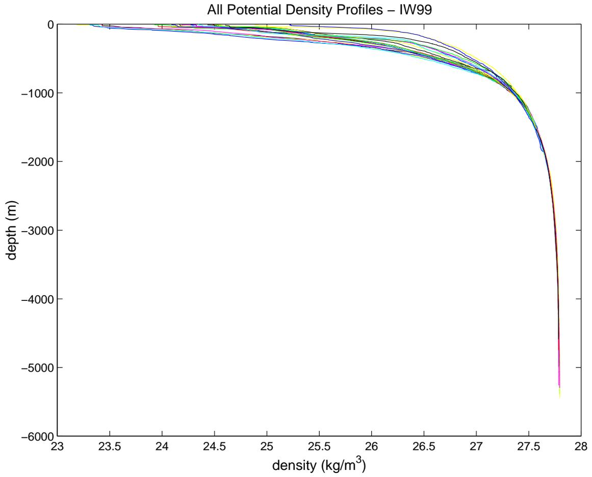
Figure 58. Potential density profiles, in kg/m<sup>3</sup>, from IW99 cruise.
