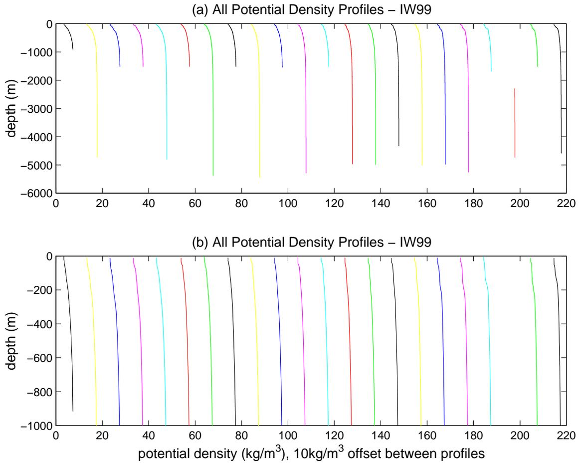
Figure 69. Potential density profiles from IW99 for (a) the entire depth and (b) the top 1000 m. All profiles separated by  $10 \text{ kg/m}^3$ .
