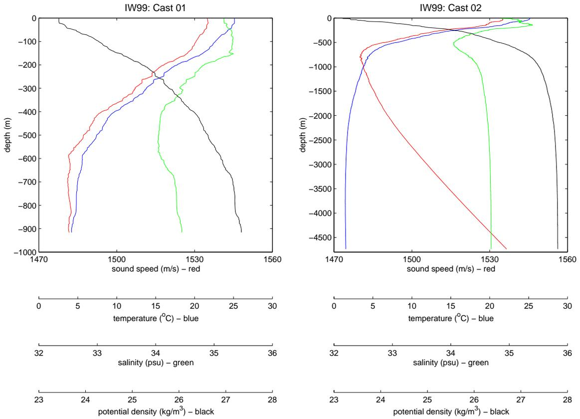
Figure 117. Processed data from Cast no. 1, file name 1701235 (left) and Cast no. 2, file name 1702114 (right) from IW99. Sound speed is in red, temperature is in blue, salinity is in green and density is in black.
