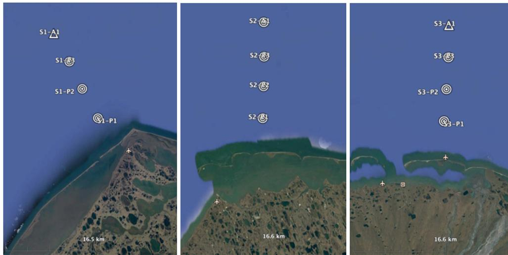
Figure 2. Detailed views of focus sites S1 (Icy Cape), S2 (Jones Islands), and S3 (Flaxman Island). Each site has an array of four moorings. Farthest offshore are A1 moorings with acoustic Doppler profilers. Farther inshore are pressure gages P3, P2, P1.
