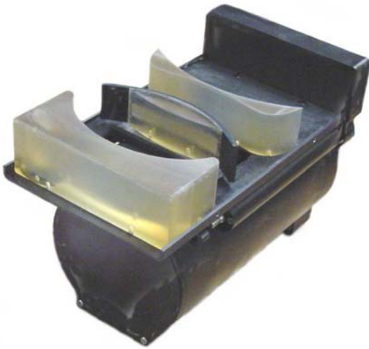
Fig. 9. DIDSON with the lens housing removed. The middle plastic lens moves fore and aft to change focus. The transducer array at the back of the lens both transmits and receives sound through the lenses. When the sonar is submerged, ambient water surrounds the lenses and transducer array.
